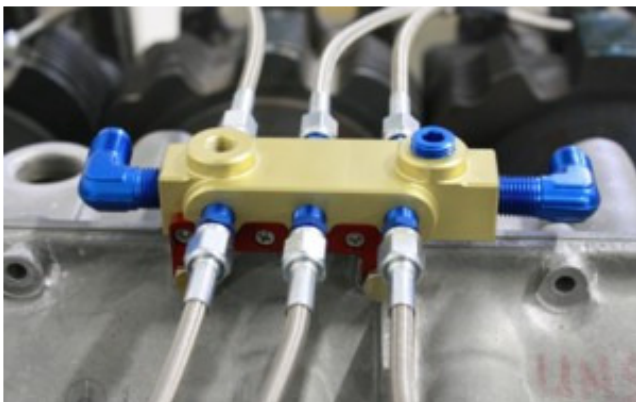
Top engine mount fuel block
