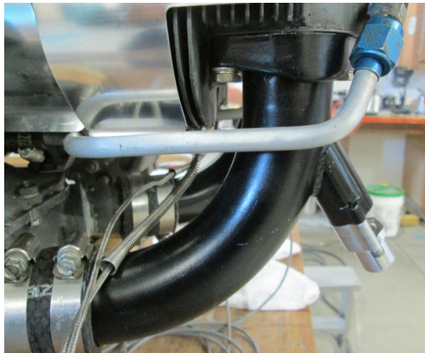
Injector boss welded in place ( Lycoming)
