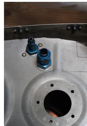
Return line using Earls Stat-o-seals
